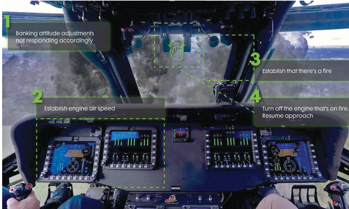
Northrop Grumman's prototype AI assistant will help rotary pilots perform expected and unexpected tasks such as augmenting the crew's response to an engine fire in this example
